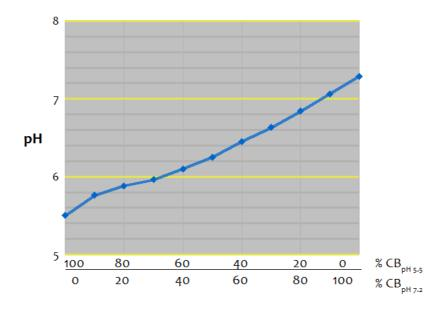
Fig. 1: pH resulting from different mixing ratios of 10x CB <sub>pH5.5</sub> and 10x CB <sub>pH7.2</sub>.
