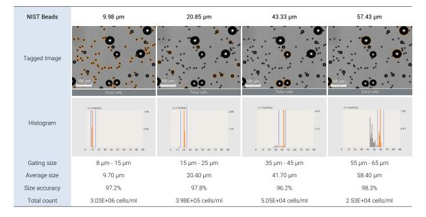
Figure 3. Specific size gating in the LUNA-FX7<sup>™</sup>. The tagged images and the histograms show that the target size particles, indicated in orange, are intensively, selectively, and exclusively detected by gating.
