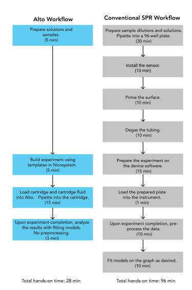
Figure 4: Flow chart of Alto vs conventional SPR workflow with step time summary. This figure summarizes side by side user workflow steps executed from sample preparation to data analysis. Overall, the same experiment required 28 minutes of hands-on operator time with Alto, instead of 96 minutes with the conventional SPR instrument.
